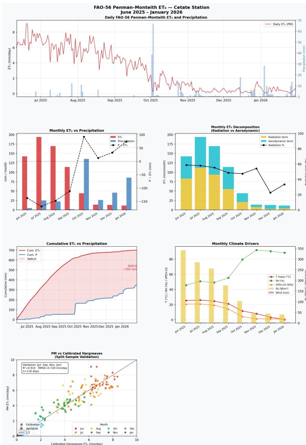
Figure 2-16 FAO-56 Penman-Monteith ET_0 analysis, Cetate station (June 2025–January 2026). Top (full width): daily ET_0 (red line) and precipitation (blue bars). Centre-left: monthly ET_0 vs precipitation with cumulative P-ET_0 deficit. Centre-right: monthly ET_0 decomposition into radiative (yellow) and aerodynamic (teal) components with radiation fraction (%). Bottom-left: cumulative ET_0 and precipitation with deficit shaded. Bottom-right: monthly climatic drivers (mean temperature, relative humidity, VPD, solar radiation, wind speed). Bottom row: Hargreaves-Samani vs FAO-56 PM ET_0 calibration scatter (split-sample validation, R^2=0.919 , RMSE=0.73 mm day -1 , n=116 days).
