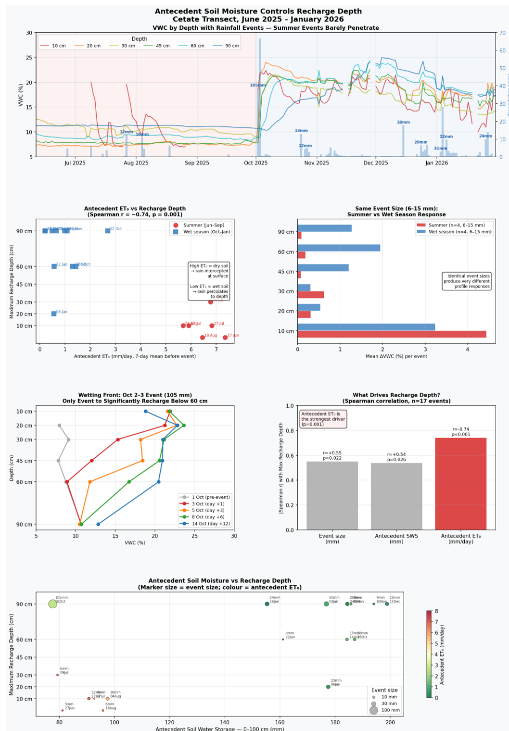
Figure 3-17 Rec threshold analysis for 17 rainfall events (June 2025–January 2026). Top (full width): VWC time series at all six depths with individual event rainfall totals annotated; summer events (barely penetrating) vs wet-season events (deep recharge) visible. Centre-left: maximum recharge depth vs antecedent 7-day mean ET_0 (Spearman r = -0.740 , p = 0.001 ; summer = red, wet season = blue). Centre-right: mean \Delta VWC per event comparing matched event sizes (6–15 mm) between summer and wet season, showing identical rainfall produces very different profile responses. Bottom-left: wetting front depth profiles for the October 2–3 event (5 dates: pre-event, peak, day +3, day +6, day +12). Bottom-right: Spearman correlation with maximum recharge depth for three predictors (event size, antecedent SWS, antecedent ET_0 ). Bottom (full width): antecedent soil water storage vs maximum recharge depth bubble scatter (marker size = event rainfall; colour = antecedent ET_0 ).
